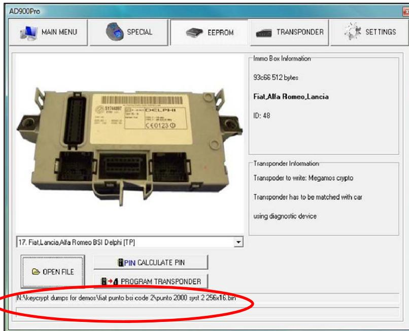
E. Click **Calculate Pin**, which will provide you with the pin code.
