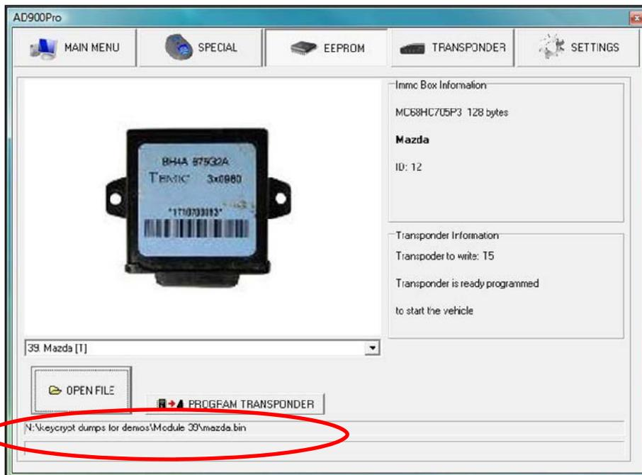
E. Insert a T5 transponder in the AD900Pro and click this option to program a transponder. You can now take this transponder, fit it into a key and start the car.
