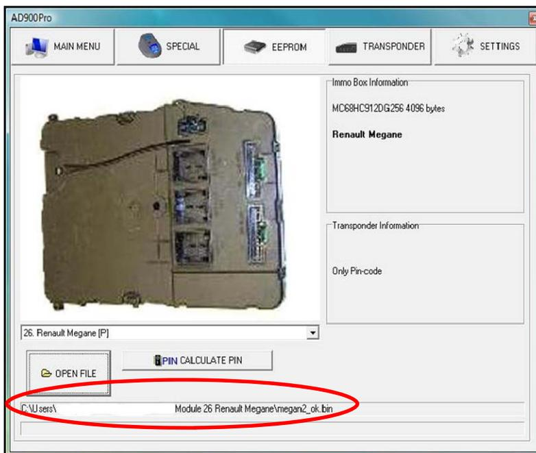
E. Click **Calculate Pin Code**. This will provide you with the pin code, that can then be used to program the key into the vehicle using a key programming tool eg AD100Pro.
