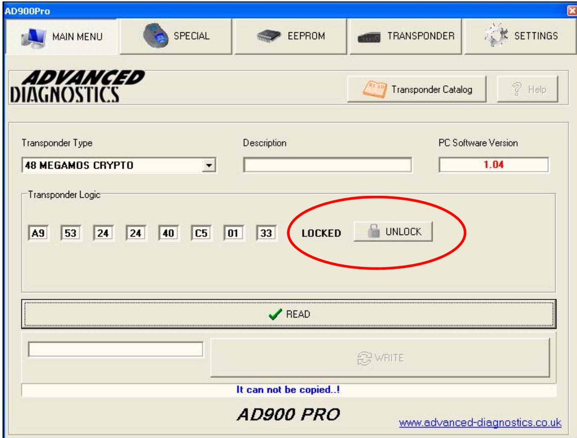
B. If the transponder is Locked it will be indicated and an **UNLOCK** button will appear.
