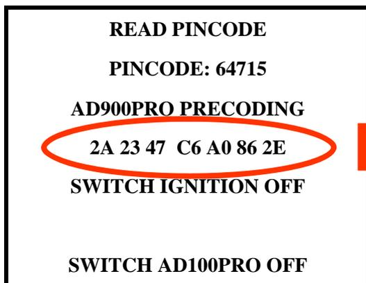
THIS IS THE 7 BYTES OF DATA REQUIRED FOR PRE-CODING THE CAN TRANSPONDERS.
