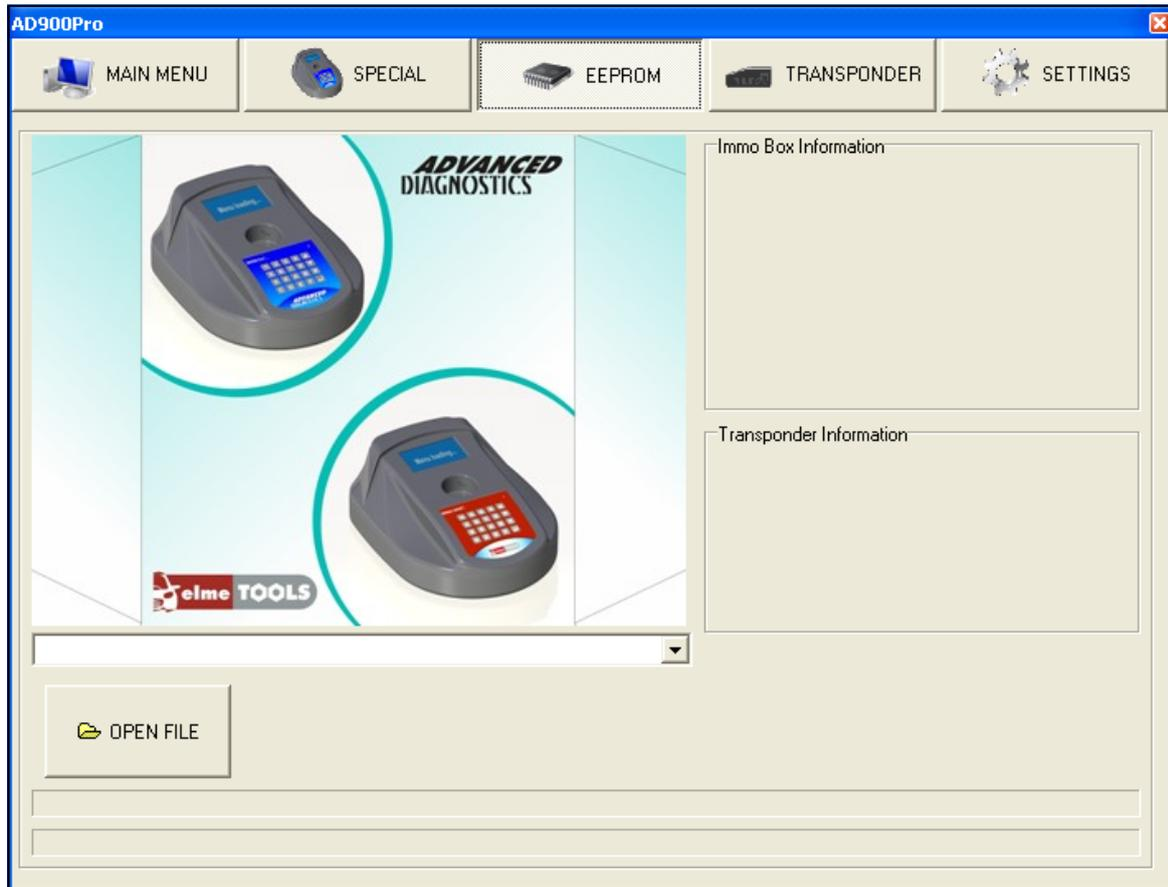
This function is used in conjunction with an EEPROM reader (not sold by Advanced Diagnostics). Depending on the system the transponder information and/or the pin code can be read.
