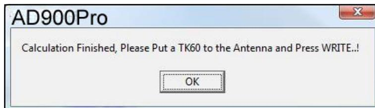
Remove the original key, place the TK60 into the reading area and Click **OK**.
