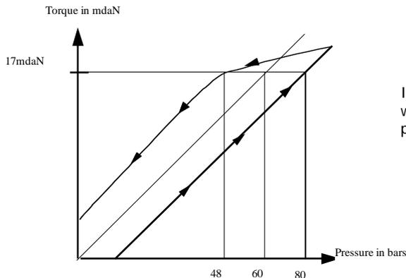
In this way (see graph), when pressure is put on the brake pedal, with a Beringer caliper a torque of 17 mdaN can be obtained with a pressure of 66 bars, instead of 80 on a standard system.
